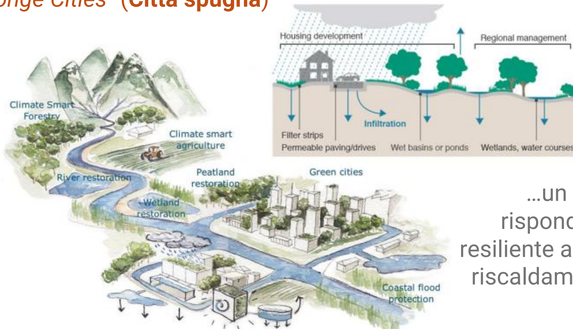
Fig. 11 The upper-right picture shows a cross-section view of SuDS (Source: https://www.susdrain.org ), the lower-left picture schematically shows the "Sponge Cities" concept, adapted from Hattum, Blauw [65] (Credits: Natasha de Sena)
